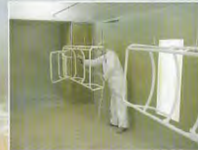
Powder coat finish electrostatically applied and baked on.
