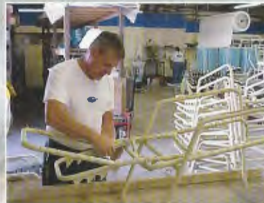
Examine for structural integrity. Replace pivots, bolts and spacers.
